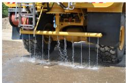
Our rear dribble bar penetrates pressurized water onto the ground. The water is fed directly from the bottom of the tank.
