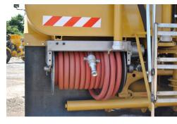
Electric Hose Reel (30 metres/100 ft of 1½″ hose with adjustable nozzle).
