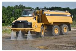
Two fully adjustable, high quality spray heads situated on a front bumper spray bar. Hydraulic or pneumatic operated from OEM supply.
