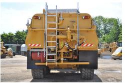
Our suction loading systems allow filling from any lakes or reservoirs. Adding this feature to your Hydex Water Tank means any source of water can be used for looking after your site. A flexible hose kit is provided to hook up to the suction loading system to begin filling.
